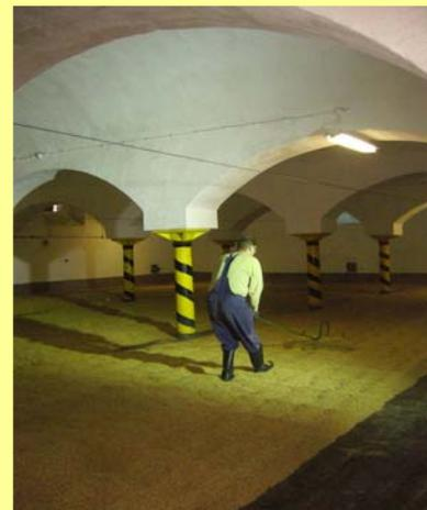
Fig. 3: Floor malt raking by „wohlgemut“ device
