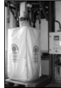
BigBag filling station
