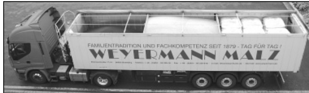
Three-chamber tractor-trailer allows for combination of bulk and bagged malt transport
