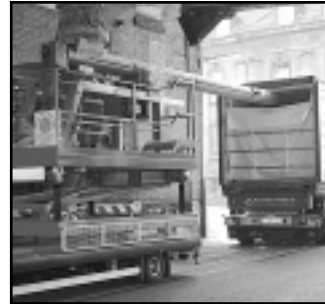
Bulk malt container loading for overseas shipments
