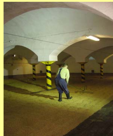
Fig. 3: Floor malt raking by „wohlgemut“ device
